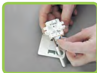
P116744 Remove the backplate and determine the position of outgoing wires (through backplate or side of cover).
