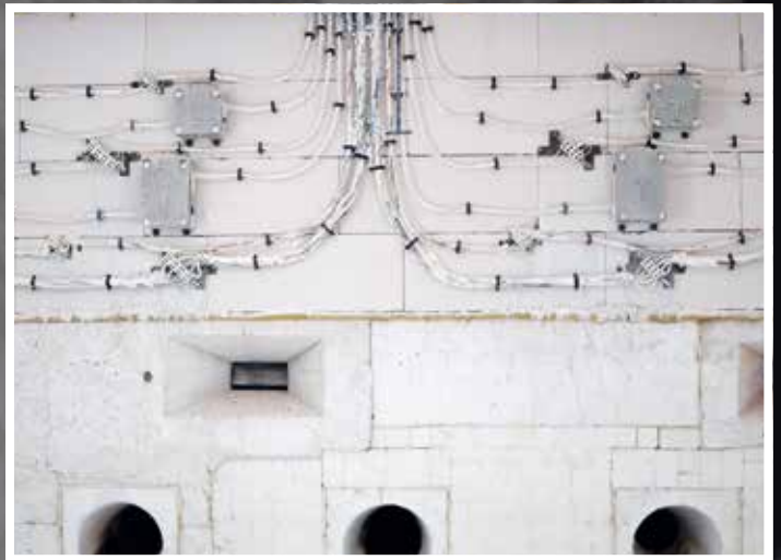
According to DIN 4102-12, the test is passed if the circuit is not disrupted for a fixed period of 30, 60 or 90 minutes.
