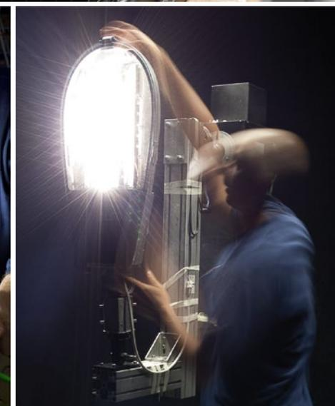
In our factory in Rezzato (Brescia), our lights are engineered, manufactured and tested. Our technical department relies on years of experience and specific instruments such as an in-house **goniophotometer** to develop optics and photometric files, an **IP and salt spray corrosion test chamber**, electrical parameters meters, **surge testers** and chromameters.
