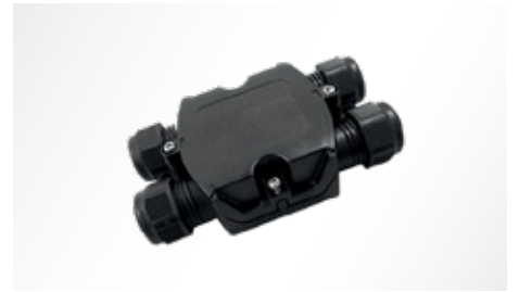
Electrical connection with quick disconnect connector in PA66 without halogens and phosphorus with silver-plated copper contacts, for cables \varnothing 9 - \varnothing 14 mm.
