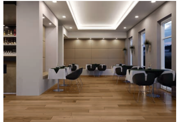
Indirect cove lighting can be used to subtly model the architecture of the room.
