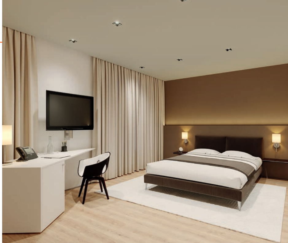
Multi-faceted lighting design in the hotel room: indirect, atmospheric over-bed lighting, supplemented by dimmable bedside lamps for reading; bright light for working at the desk.
